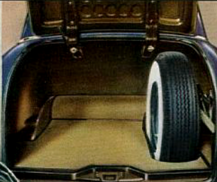
ROOMY LUGGAGE COMPARTMENT has spare tire at right, out of the way, yet easily accessible. Special lock-down stowage for bumper jack eliminates rattles.
